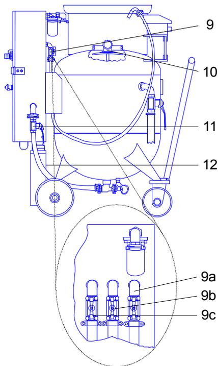
**Switching ZW (11) – Equipment (511):** It allows to switch over from blasting to cleaning or to drying at the machine.
